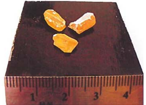
Single Crystal Piezoceramics, grown by Lasergenics, Inc., will be used as base material for large-displacement actuator stacks.
